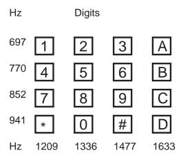
The tone-dialing method combines two frequencies for each of the twelve digits found on a Touch Tone dial pad. This method is referred to as Dual-Tone Multi-Frequency (*DTMF*) dialing. The four horizontal rows on a Touch-Tone keypad use the four low frequencies (697, 770, 852, 941 Hz), while the three vertical columns use the three high frequencies (1209, 1336, 1477 Hz). The generally accepted tone frequency tolerance is +0.02%.
